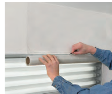
Using a SNIPPET KNIFE or razor blade, cut across film at top edge of lightbox. (Do NOT cover lightbox*.)
